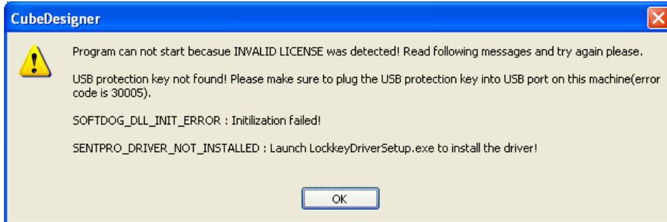
Figure 3 Error message on missing lock key
